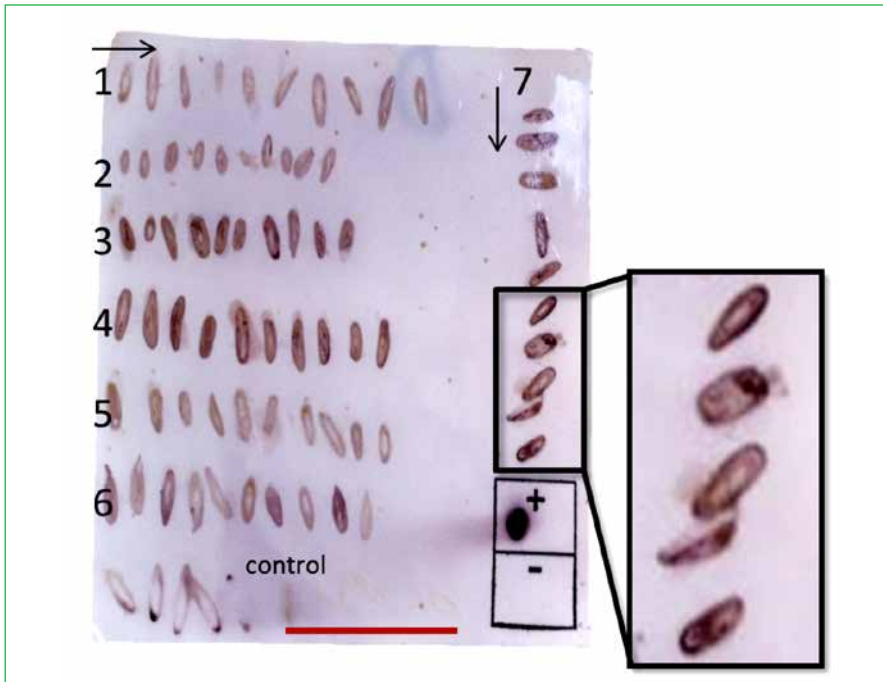
Plate 1: Nitrocellulose membrane imprinted with the extracted Neotyphodium endophyte proteins. The insert shows the imprint of endophyte infected seeds clearly defined as dark colour development. Light colour developments are negative. The subjective output of this test is illustrated here. Seven different cultivars with ten replicates are imprinted here. There are five negative seeds on this membrane underlined in red; these are the known uninfected control seeds.
