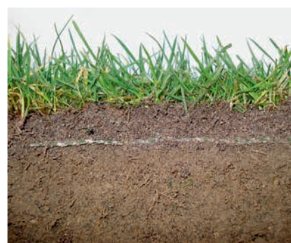
Fig. 3: Hybrid turf system PowerGrass: stabilization mat in the root zone, filled with 2.5 cm root zone mix.
