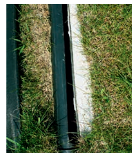
Fig. 2: Slit ABS pipe placed at the lowest part of the plots to collect runoff water.
