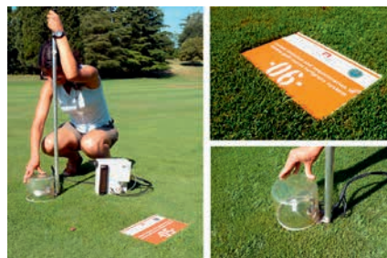
Fig. 1: Measurement during field survey; portable IRGA-EGM4 (PP Systems, UK), connected to a custom chamber, and iron plates marking NEE measurement points.
